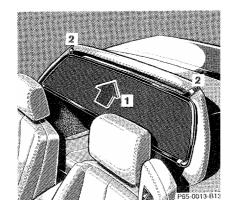
3. Slide wind screen up into roll bar (1), using care not to get the attachment straps (2) caught.
