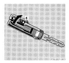
Change batteries, inserting new ones under contact spring (5) with plus (+) side facing up.
