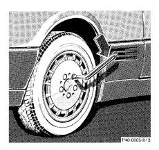
Observe a tightening torque of 80 ft. lb. (110 Nm).
