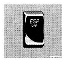
ESP control switch located in center console
