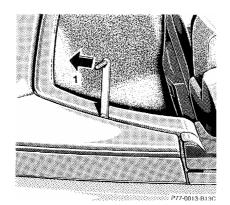
Unlock left and right soft top storage compartment locks: Place open-end wrench on bolt between roll bar and storage compartment cover. Turn wrench towards rear of car (1).
