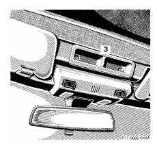
If the soft top switch is held or is released and slid forward again within approx. 2 seconds, the side windows will close. If the roll bar was previously in the upright position, it will return to that position.
