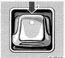
Please note, if soft top switch is activated after 10 seconds have expired, turn the key back to position 0 first before the hardtop removing procedure can be started again at step 4.
