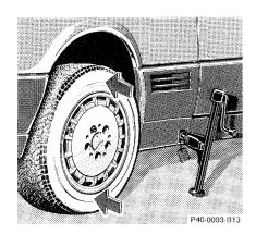
Clean contact surfaces of wheel and wheel hub. Install spare wheel on wheel hub. Insert wheel bolts and tighten them slightly.
