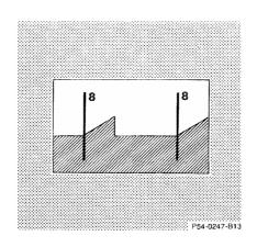
7. The indicator (7) in the sight glass should align with the "0" mark after any horizontal adjustment. If it does not, insert and turn screw driver on adjuster (3) until scale (7) is centered on the "0" mark.
