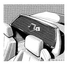
5. Pull wind screen down out of roll bar (5) and lift wind screen out on one side and remove.
